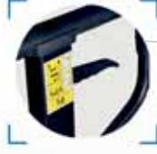
3-position (lowering - neutral - lifting) control lever in the steering arm.
